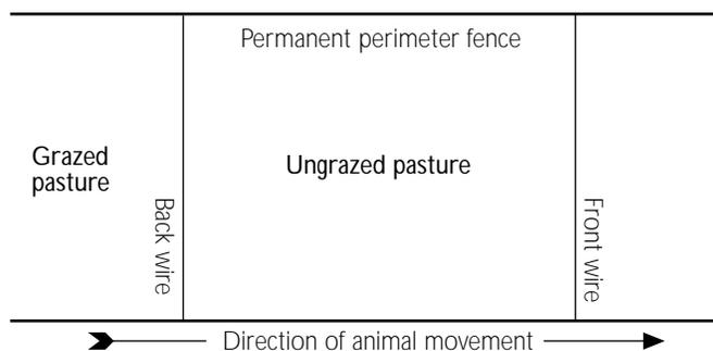
**Figure 7. Strip grazing.** The paddock has two wires which are moved along two permanent fences. Move the front wire according to pasture production and animal need. Follow with the back wire to prevent grazing of re-growth.
