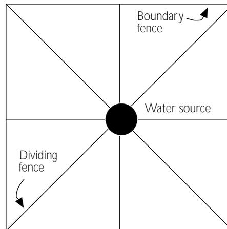
**Figure 8.** Access to a central watering site with paddocks in a "pie layout" (*not recommended*)
