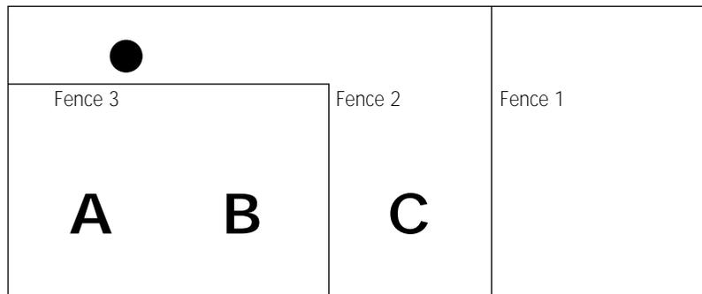
**Day 5**— Fence 1 is removed and used as the new back fence. Fence 2 is rolled up to let cattle move in; fence 3 is extended.
